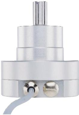
DEIF's rudder/azimuth angle transmitters convert the rudder or azimuth thruster's position angles into either electrical 4-20 mA signals or digital data values with a 16 bit resolution (+/-180deg. = +/-32767).
