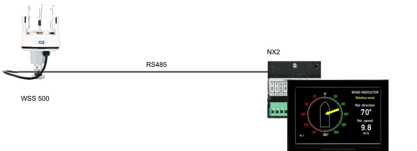
The RS485 port is used to receive NMEA data from the windsensor
